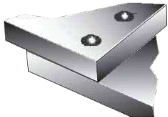
Plug Welds (Fig 1-19j)
